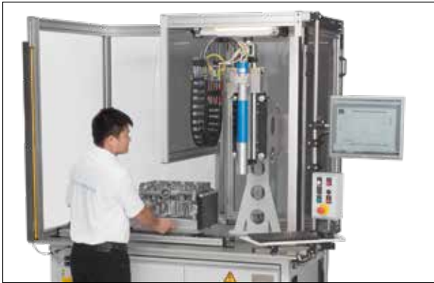
Station with manual loading for small series or prototype production
