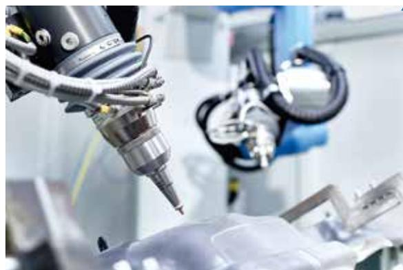
Robot-based laser machines for cutting and welding metal.
