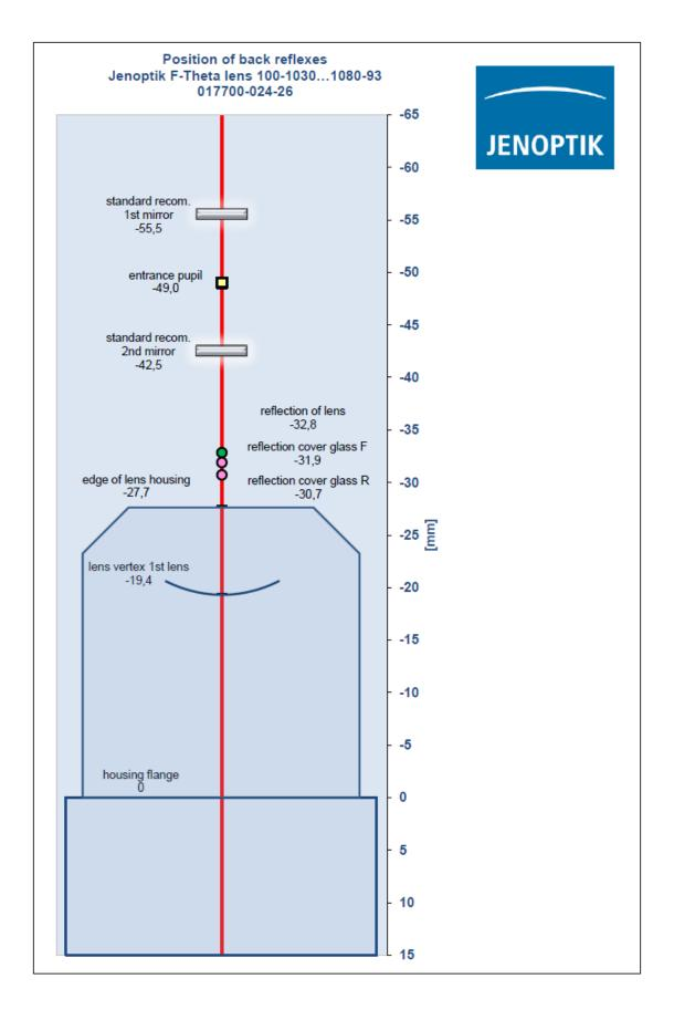
The graph illustrates all paraxial back reflection positions outside the F-Theta lens. Back reflections inside the lens are optimized to be located away from any lens surface and element. All values are only valid for collimated beams and appropriate use of this lens. Changing system settings or operating conditions can lead to varied reflex positions and cause damage.
