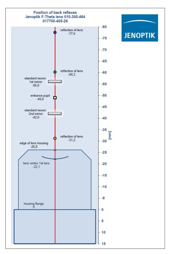
The graph illustrates all paraxial back reflection positions outside the F-Theta lens. Additional back reflection positions occur at a range of -209 to -209.7 mm.
