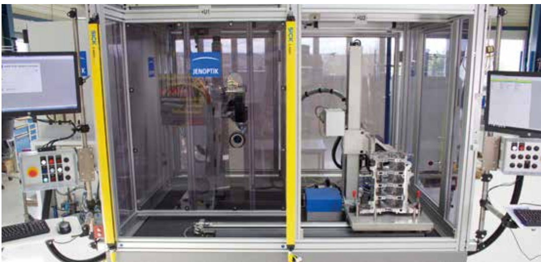
Combined cylinder inspection using B100 and CF1250
