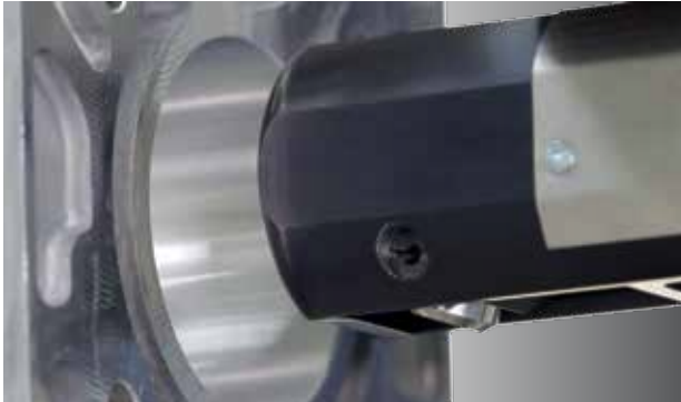
Measuring a cylinder bore
