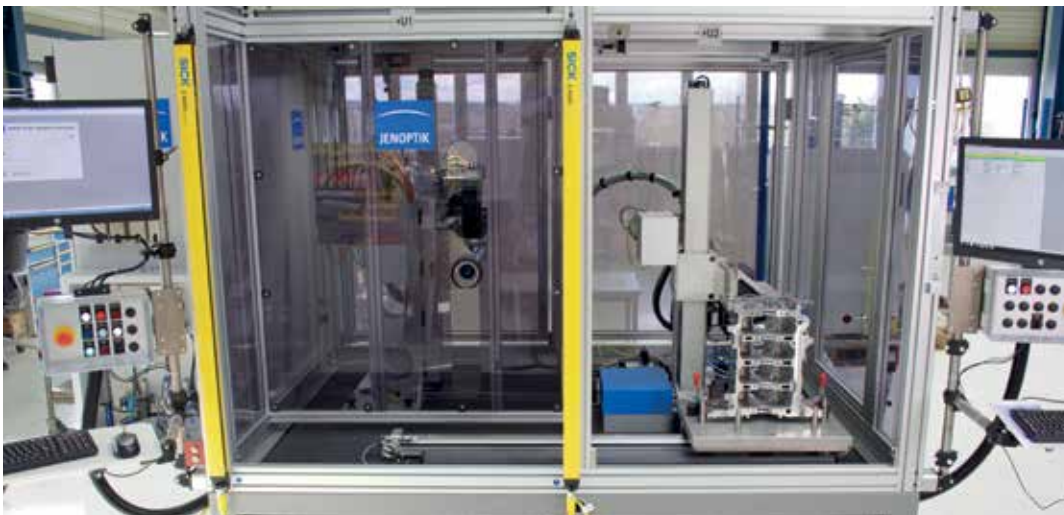
Combined cylinder inspection using IPS B100 and CCS C100
