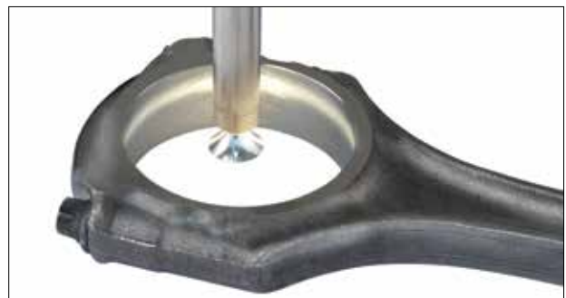
Inspecting the inner bore of a con rod eye
