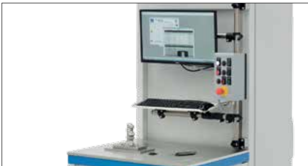
Inspection station for inspecting master cylinders
