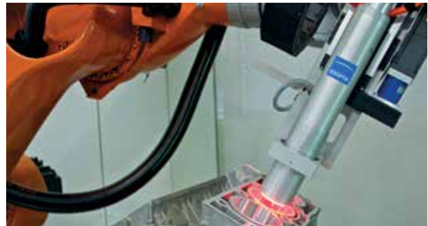
Robot-guided inspection cell
